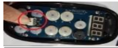
Signal cord loose/ PCB failure
